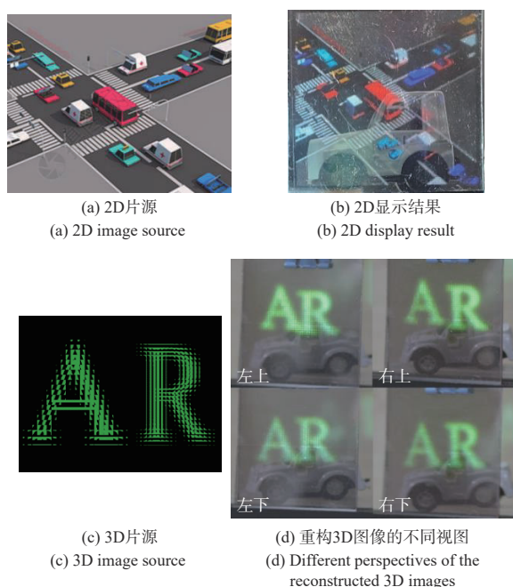
图 7 增强现实 2D/3D 兼容显示系统显示效果 Fig.7 Display results of the augmented reality 2D/3D compatible display system
